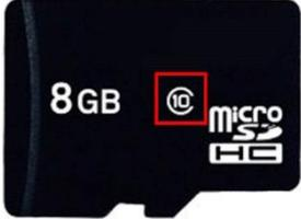
We need a **Micro SD card reader** and a **Micro SD card** with minimum of 4GB storage, we suggest the Micro SD Card to be Class 10, for faster read/write speed.
