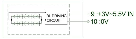
PIN10 is connected to PIN2(VSS) internally
