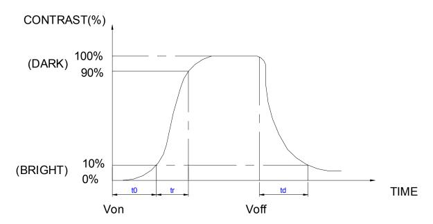
Delay time to : Measured between zero and 10% with Von.
