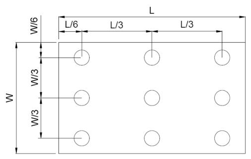
Figure 4.3 Definition of measuring points.
