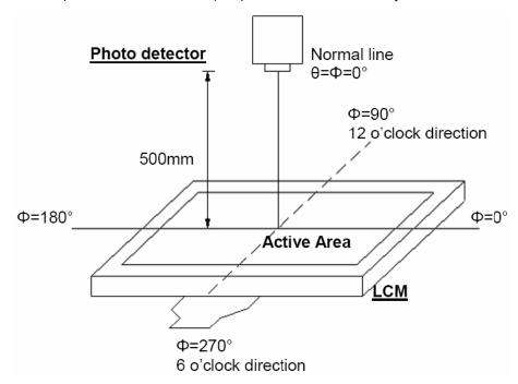
Figure 5.2 Optical measurement system setup
