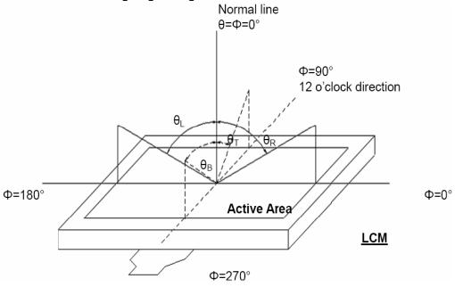
Figure 5.1 Definition of viewing angle.
