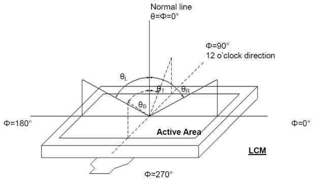
Figure 4.1 Definition of viewing angle.
