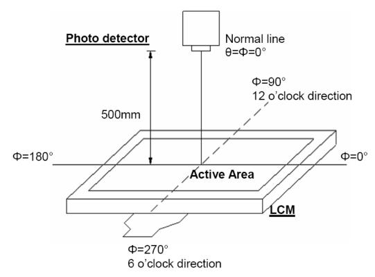
Figure 4.2 Optical measurement system setup
