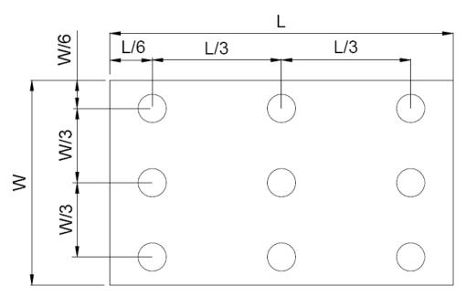
Figure 4.4 Definition of measuring points.
