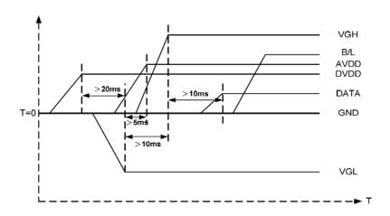
$$V_{DD} {\rightarrow} V_{GL} {\rightarrow} V_{GH} {\rightarrow} Data {\rightarrow} B/L$$
