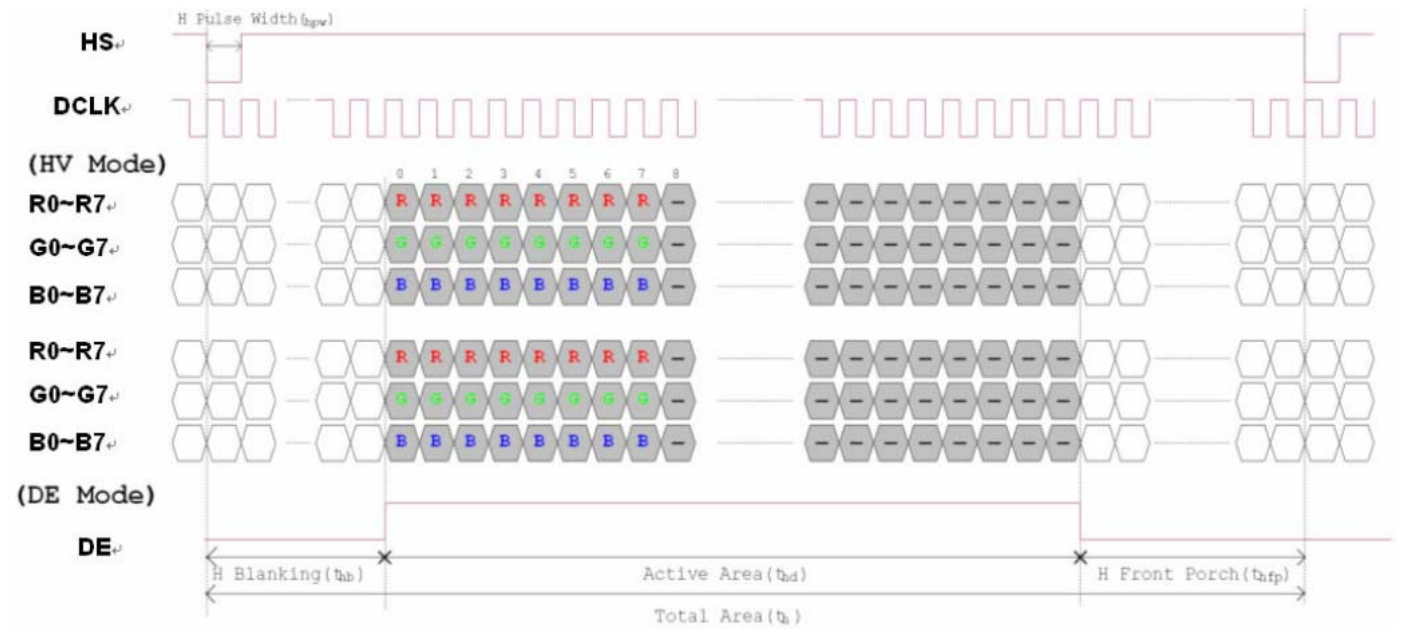
Figure 3.1 Horizontal input timing diagram.
