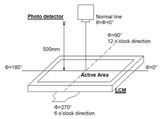
Figure 4.2 Optical measurement system setup
