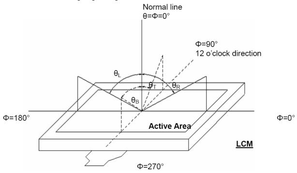
Figure 4.1 Definition of viewing angle.
