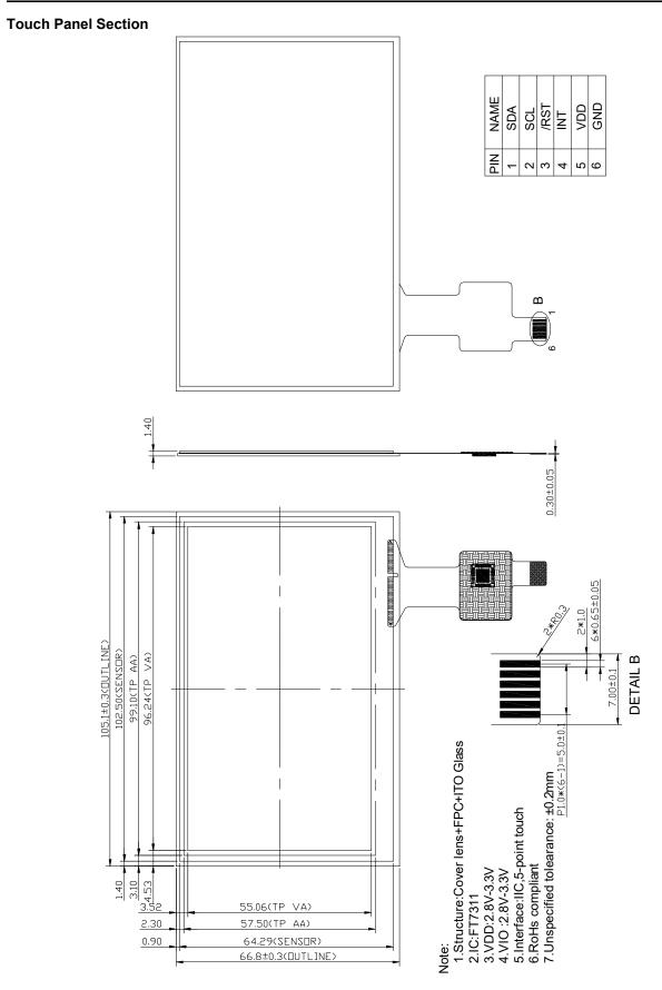
Recommended connector: Hirose FH12-6S-1SH(55) or compatible
