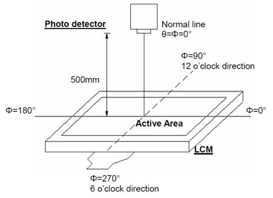
Figure 4.2 Optical measurement system setup
