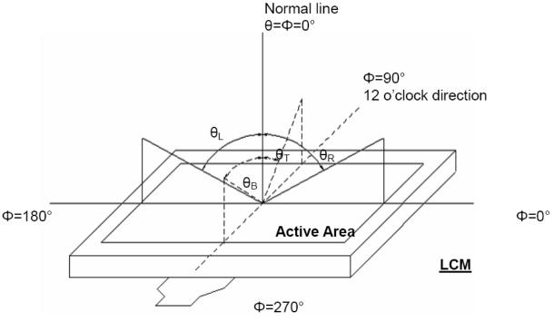
Figure 4.1 Definition of viewing angle.
