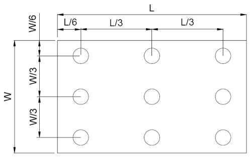
Figure 4.4 Definition of measuring points.
