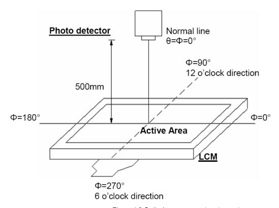
Figure 4.2 Optical measurement system setup
