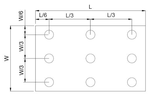
Figure 4.3 Definition of measuring points.
