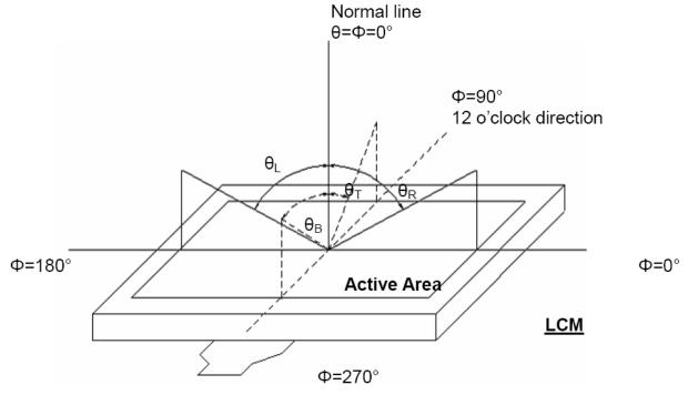
Figure 4.1 Definition of viewing angle.
