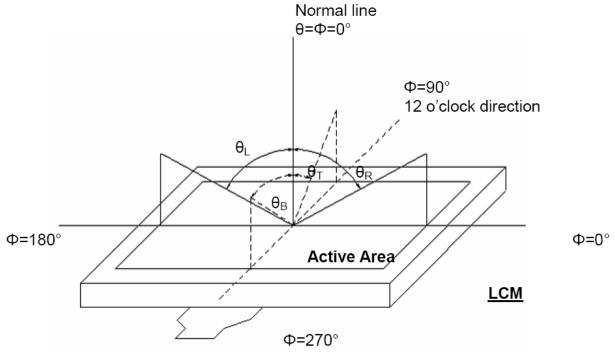
Figure 4.1 Definition of viewing angle.
