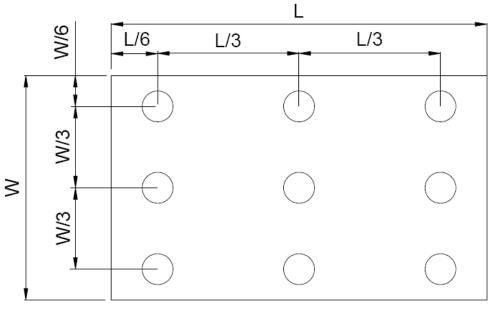
Figure 4.4 Definition of measuring points.
