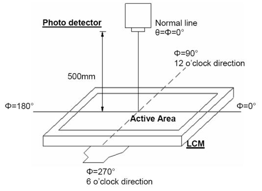
Figure 4.2 Optical measurement system setup
