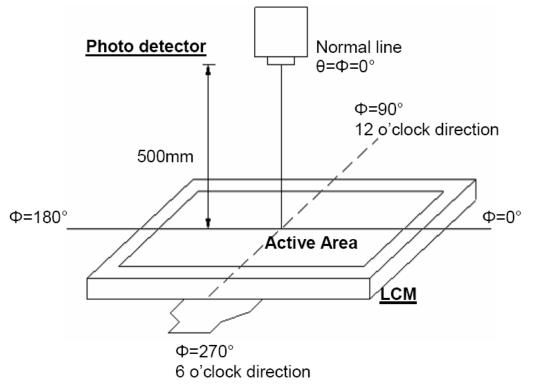
Figure 4.2 Optical measurement system setup
