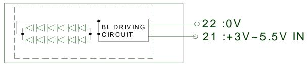
PIN22 is connected to PIN2(VSS) internally
