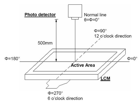
Figure 4.2 Optical measurement system setup
