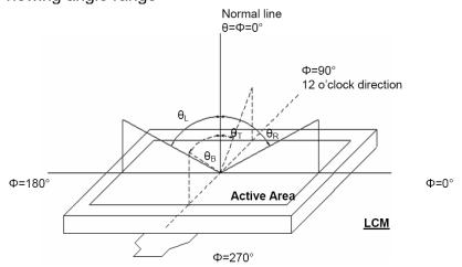
Figure 4.1 Definition of viewing angle.
