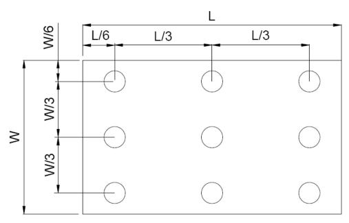
Figure 4.3 Definition of measuring points.
