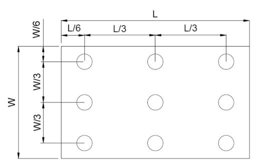
Figure 4.3 Definition of measuring points.
