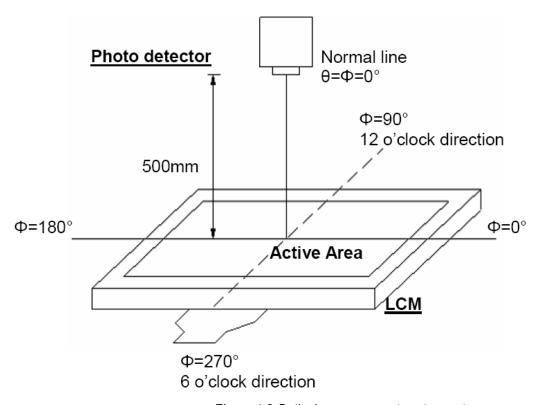
Figure 4.2 Optical measurement system setup
