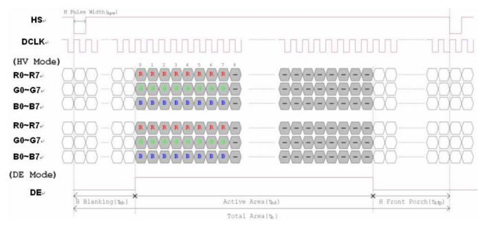
Figure 3.1 Horizontal input timing diagram
