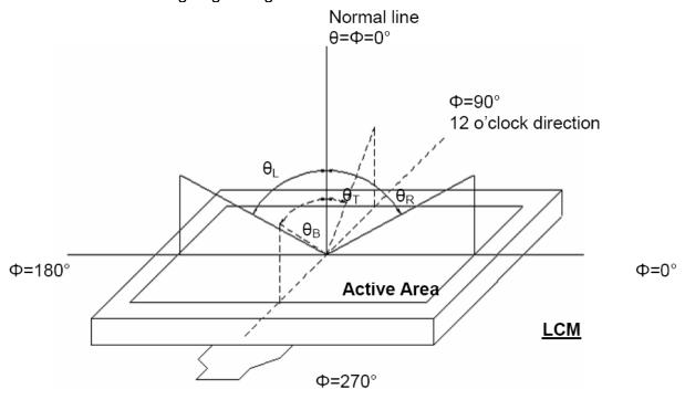
Figure 4.1 Definition of viewing angle.
