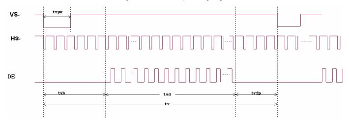
Figure 3.2 Vertical input timing diagram
